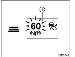
When passing another vehicle, the set speed indicator (B) will flash when the vehicle speed exceeds the set speed. The vehicle detect indicator will turn off when the area ahead of the vehicle is open. When the pedal is released, the vehicle will return to the previously set speed.
