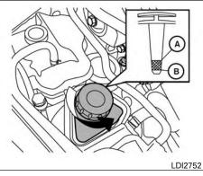
Check the fluid level in the reservoir.
