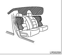
Front seat-mounted side-impact supplemental air bag and roofmounted curtain side-impact and rollover supplemental air bag systems
