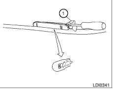
**Step light (if so equipped)** Use a cloth ① to protect the housing.
