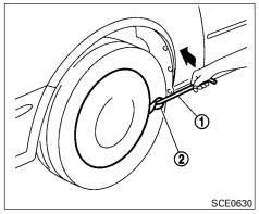
Removing wheel cover (if so equipped)
