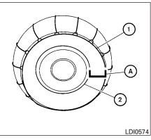
Use of tire chains may be prohibited according to location. Check the local laws before installing tire chains. When installing tire chains, make sure they are the proper size for the tires on your vehicle and are installed according to the chain manufacturer's suggestions. Use a tire chain that is designed to provide the specified space (A) between the installed tire chain (1) and where the tire meets the rim (2) as shown on the chart.
