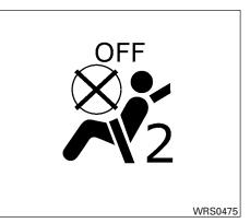
If the booster seat is installed in the front passenger seat, place the ignition switch in the ON position. The front passenger air bag status light may or may not illuminate, depending on the size of the child and the type of booster seat being used. For additional information, refer to "Front passenger air bag and status light" in this section.
