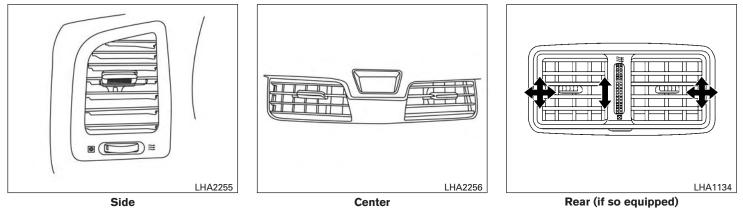
Adjust air flow direction by moving the vent slides.
