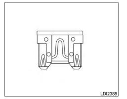
If any electrical equipment does not operate, check for an open fuse.
