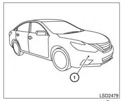
The PFCW system uses a radar sensor (1) located on the front of the vehicle to measure the distance to the vehicle ahead in the same lane.
