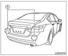
The BSW system uses radar sensors (1) installed near the rear bumper to detect other vehicles in an adjacent lane.
