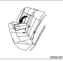
To fold down the driver's side of the rear seat, open the trunk and pull on the strap 1.
