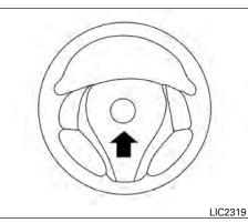
To sound the horn, push near the horn icon on the steering wheel.
