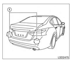
The RCTA system uses radar sensors 1 installed on both sides near the rear bumper to detect an approaching vehicle.
