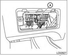
3. Remove the fuse with the fuse puller  $(\mathbf{A})$ .
