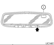
Press the -N- button for about 1 second when the ignition switch is placed in the ON position to toggle the compass display ① on or off. The display will indicate the direction of the vehicle's heading.
