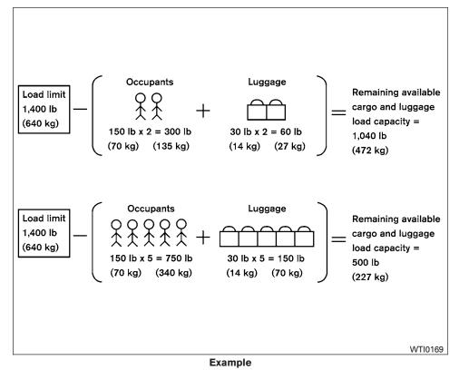
Steps for determining correct load limit
