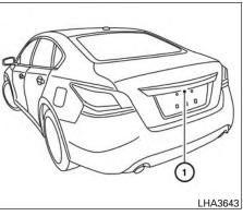
To display the rear view, the RearView Monitor system uses a camera located just above the vehicle's license plate (1).
